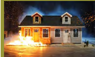
Figure 2b Embers impacting a building; left side with combustible (wood) and the right with noncombustible (rock) mulch.
