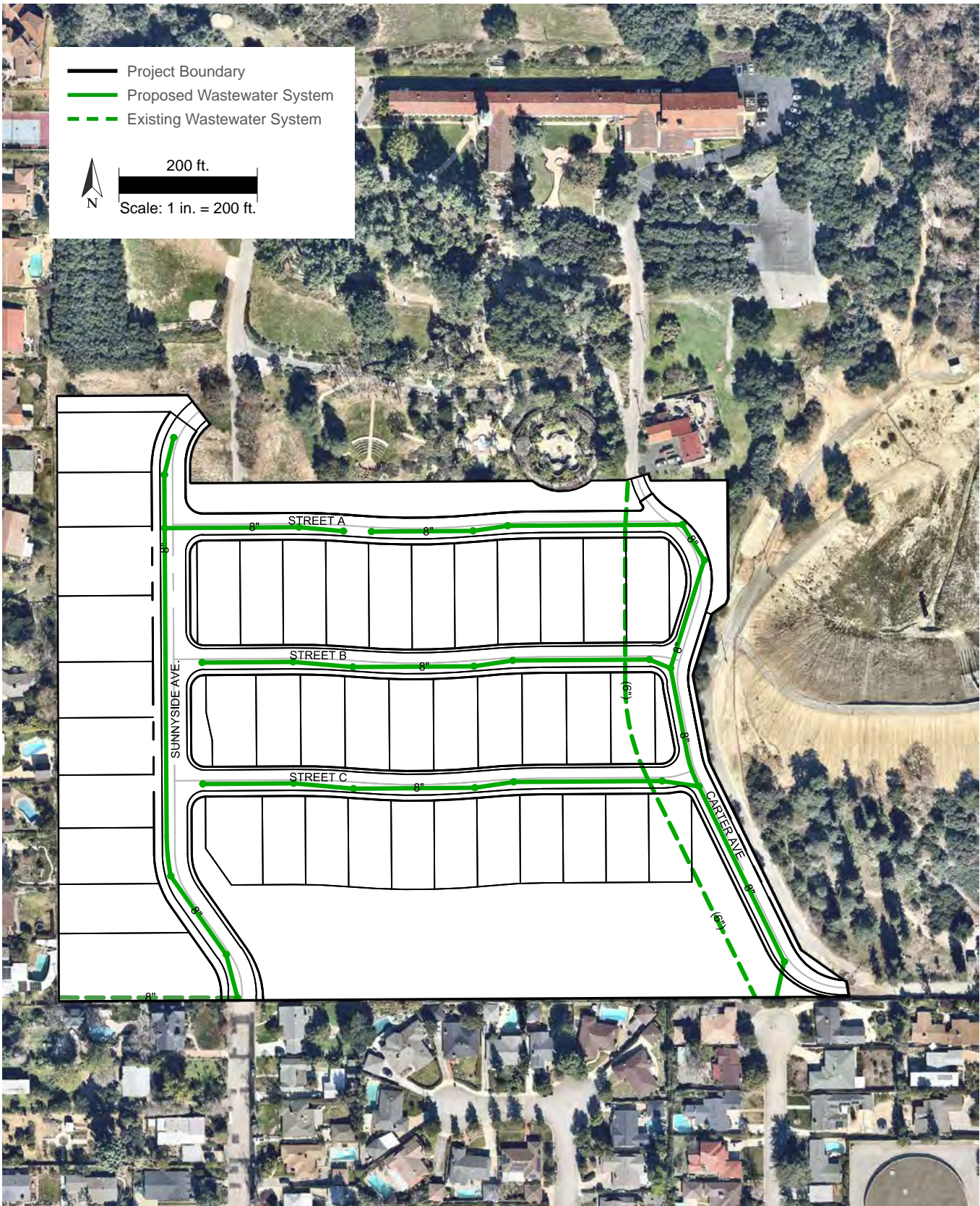
Figure 4-8: Existing and Proposed Wastewater System
