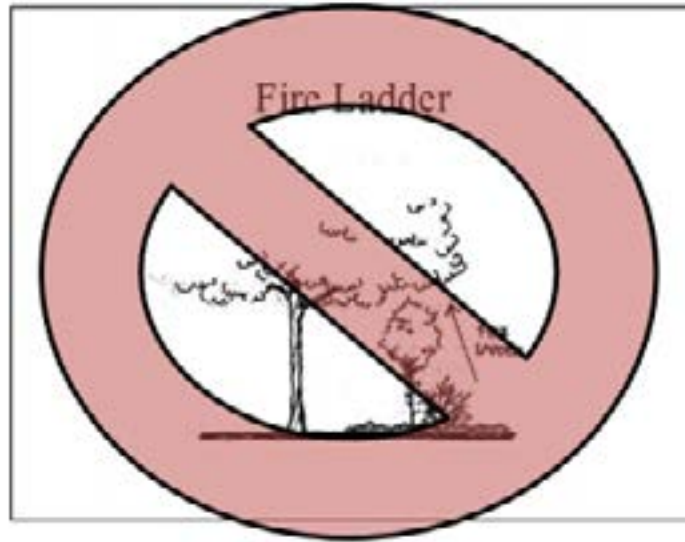
Figure 1: Fire Ladders or Fuel Ladders should be eliminated. The diagram above illustrates what not to do.
