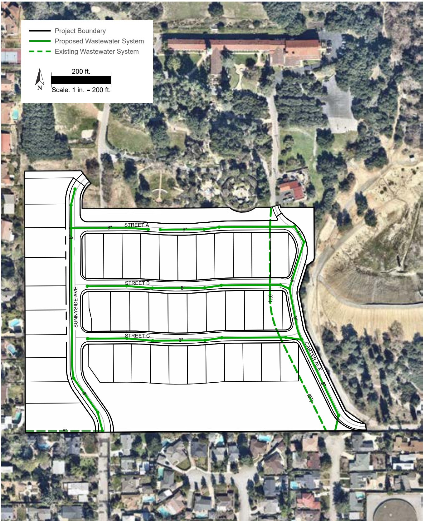
Figure 4-8: Existing and Proposed Wastewater System
